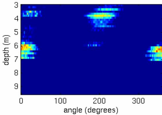
Figure 4 Reflectivity (90% clip) of field data over the whole data volume. Note that, an object is observed at 6.4 m depth and at 350 degrees. The accuracy can be improved by verifying B-scans.
