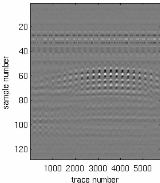
Figure 2 Laboratory data. The x-axis is the trace number, representing depth, since the radar moves from 4m to 1m depth while measuring traces. The number of traces per depth scan is 256.
