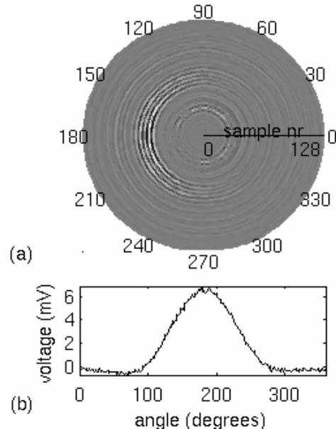
Figure 3 Angular view of the laboratory data shown in Figure 2. (a) One common-depth scan at depth of object which is located at 180 degrees in angular direction. (b) Sample 58 of this common-depth scan.
