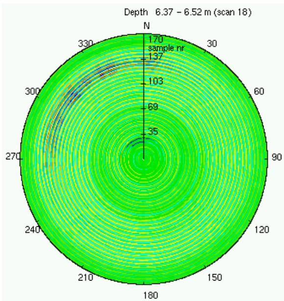
Figure 5 Field data, muted and mean depth scan subtracted. Shown is a depth scan at the depth of the object. The numbers around the scan denote the angle. The object is located at 330 degrees. Only the first 256 samples are shown.
